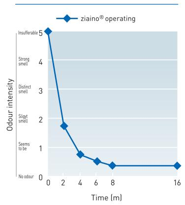
The mean value of odour intensity was calculated after removing 1 maximum value and 1 minimum value from the judgment values of 6 sniffers.
